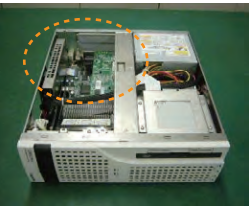
EMC Gaskets on the Expansion Bus Slot's Window ➡
