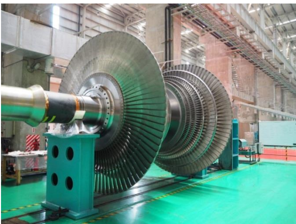
800MW super-critical LP turbine rotor for Kudgi Unit 2
