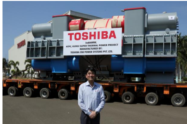
Toshiba’s First ‘Made in India’ 800-megawatt steam turbine and generator (STG) for Unit 2 of NTPC’s Kudgi Super-critical Thermal Power Station
