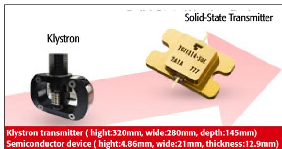
Klystron transmitter ( height:320mm, wide:280mm, depth:145mm)
